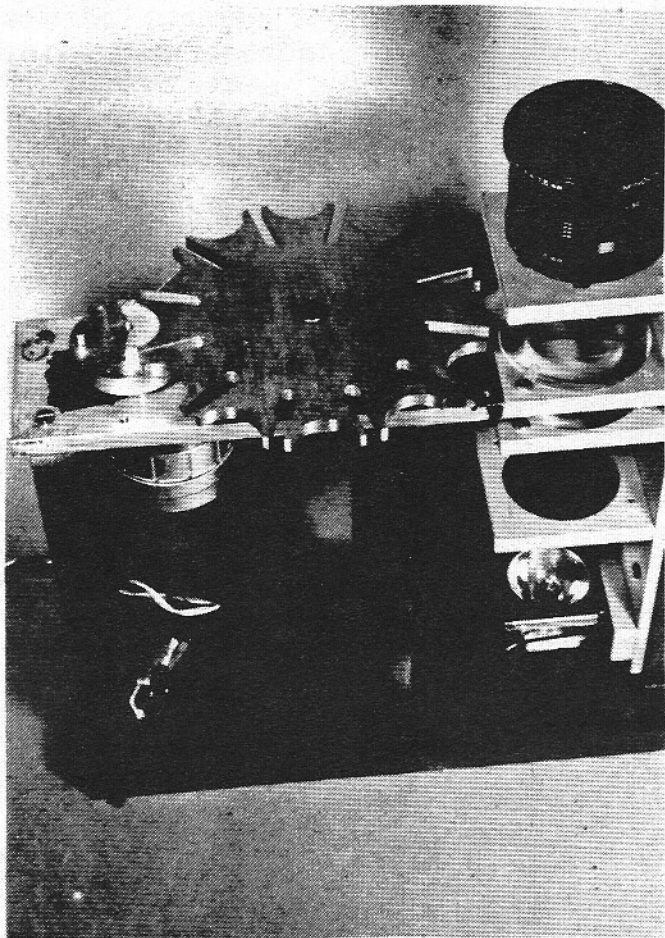
Figure 2: All-Sky projector with slide plate removed to show Geneva movement (slotted, scalloped wheel)
